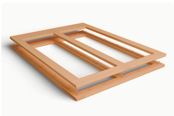
Rear layer lifted for clarity; assemble flat on a protected caul.
